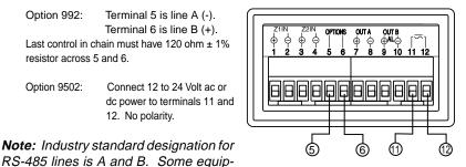
ment manufacturers use a non-standard designation of plus and minus. association of A to minus and B to plus is based on a sample of devices marked as plus and minus and is not intended to represent ALL such labelled devices. Final responsibility for correct identification of leads and terminals rests with the user/ installer and the manufacturer of the other device(s) installed in the system.
